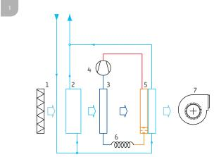
Schematization of an isotherm dehumidifier.
