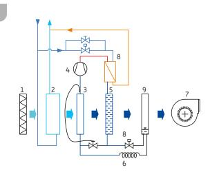
Schematization of a sensible integration dehumidifier.
