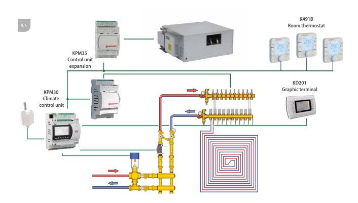
be defined and associated to each thermostat. The display-free version of the KPM31 control unit can be combined to the KD201 graphic terminal as programming interface.
