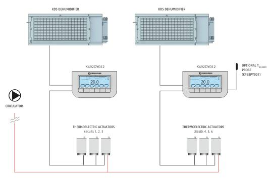
Connection diagram for K492DY012 with thermoelectric actuators and dehumidifiers
